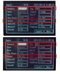
3 After the setting is completed, the measured values of the analog quantity can be read through the PLC. Channel 1 is the temperature value, and channel 2 is the dew point value (as shown in the following figure):
