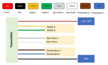
Please check the transmitter wiring to prevent damage to the transmitter due to incorrect wiring! Please wire transmitters with different analog output types according to the diagram below.
